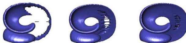
Fig. 20. Effect of the resolution on the surface at t = 1 : h = 1/100 , 29,073 particles (left), h = 1/160 , 94,033 particles (middle), and h = 1/200 , 169,500 particles (right).
